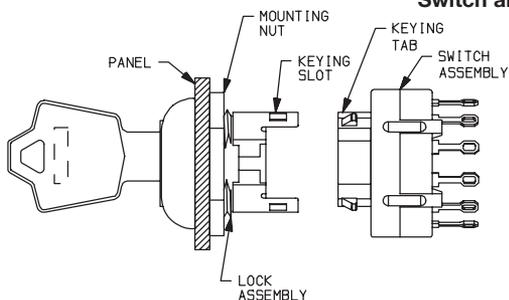
1. Place lock assembly in mounting hole on panel, secure with mounting nut.
