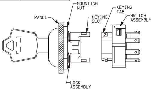
1. Place lock assembly in mounting hole on panel, secure with mounting nut.
