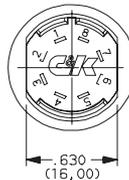
Terminal numbers molded on bottom of housing.
