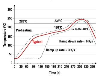
Soldering process: Depending on the application, this component is suited to the following methods:
